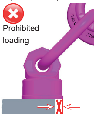
Pic. 3: The diameter of the bearing surface must be \geq D
