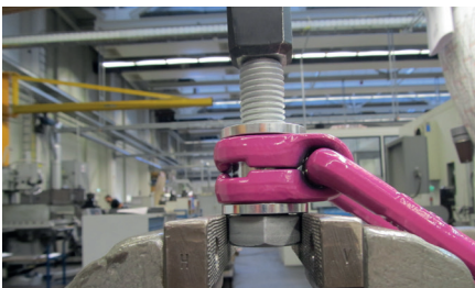
Pic. 7: Dismantling position of the VLBG
